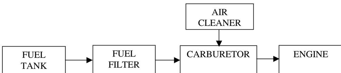
**Fuel Tank** - It is reservoir of fuel oil for an engine. It is kept in an elevated position so that the fuel will flow to the carburetor through the filter by gravity. Our fuel tank has a capacity of 1 litre and there is also a fuel level indicator in it.
