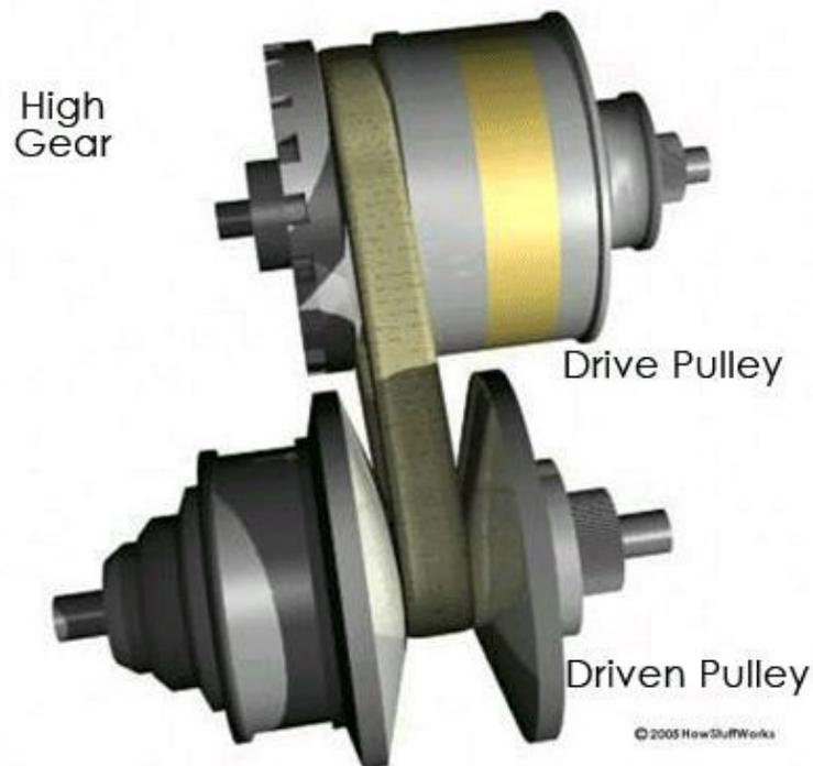
The distance between the centers of the pulleys to where the belt makes contact in the groove is known as the pitch radius. When the pulleys are far apart, the belt rides lower and the pitch radius decreases. When the pulleys are close together, the belt rides higher and the pitch
