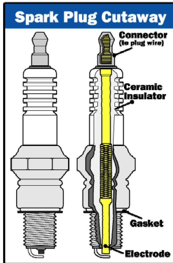
The central electrode is seated into the insulator and is provided with a screwed terminal at the upper exposed end, often shaped to accept a snap-on connector. The tip of the electrode, at which the spark occurs, usually has an insert of heat-resisting metal such as nickel.
