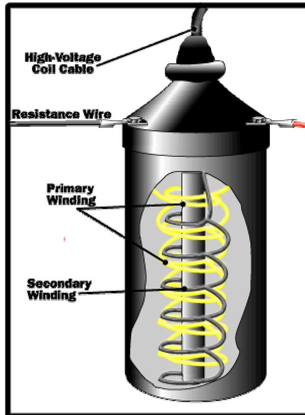
The voltage required to cause a spark between the sparking plug points depends upon both the pressure of the mixture with the cylinder and the gap between the points under average conditions a voltage of the order of 10,000 volts is needed.
