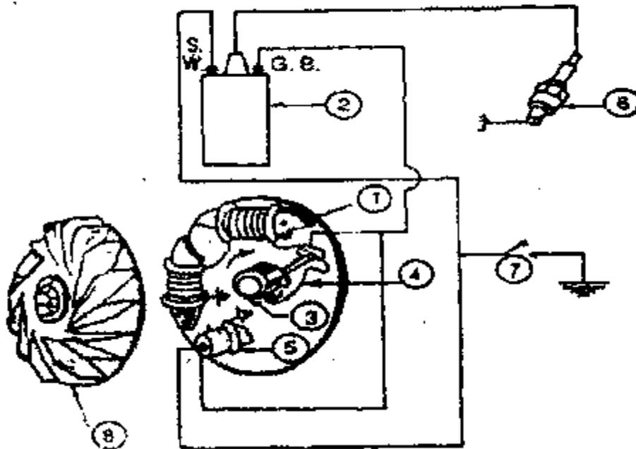
FLY WHEEL MAGNETO (ROTATING MAGNET TYPE)
