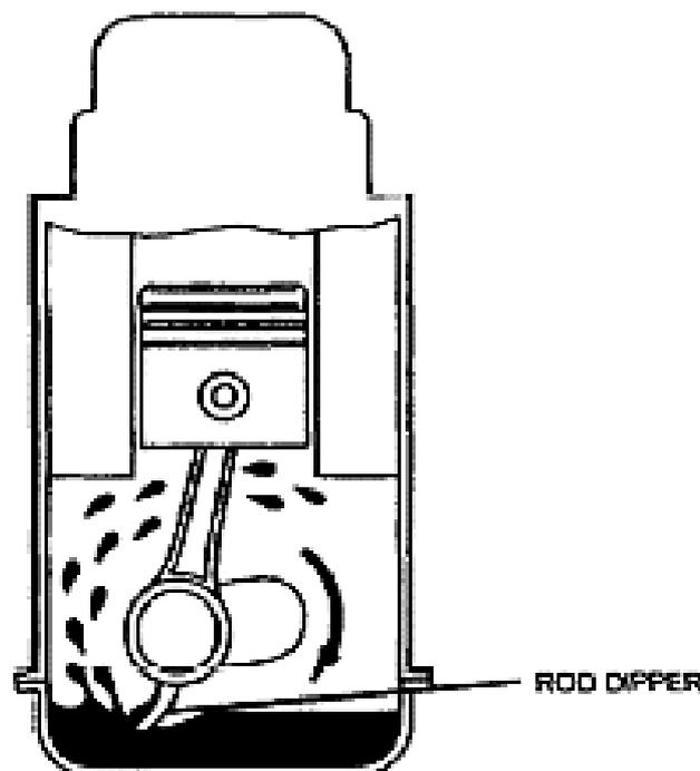
The splashed oil is in the form of a dense mist sprayed into fine particles over surfaces in contact. Small cups are provided close to the bearing of the crankshaft. There are small holes in these cups. The splashed oils fills up these cups from where it is supplied to the bearing.
