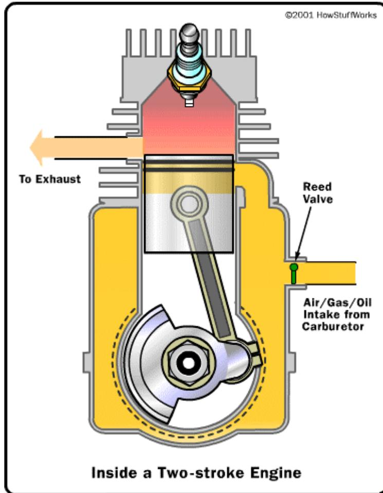
The pre-compressed fuel-air mixture travels from the crankcase to the combustion chamber through the transfer port. The fresh fuel air mixture is fed into the combustion chamber with the help of a deflector on the piston head. It guides the mixture through the transfer port into the combustion chamber towards its top.
