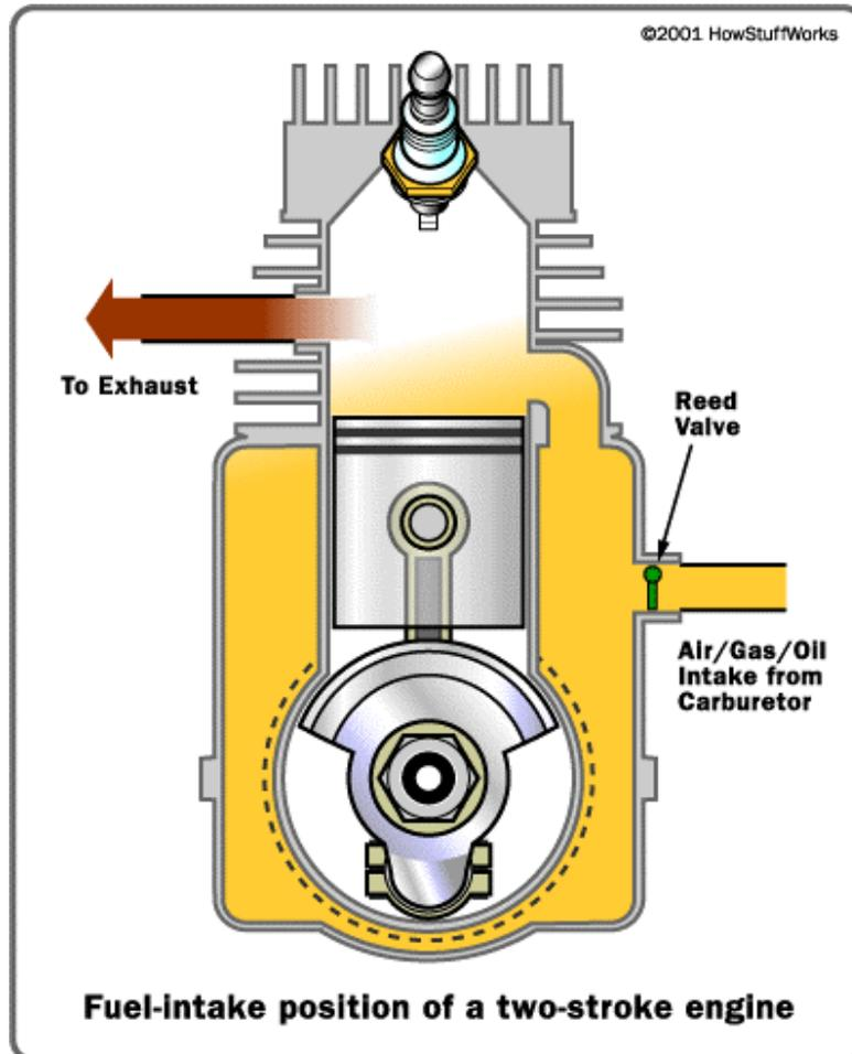
In this process, the piston uncovers the inlet port. Fresh charge of fuel-air mixture enters the crankcase owing to vacuum produced in it. This is due to the upward movement of the piston. Thus, in one stroke of the piston, two operations, via suction and compression are carried out. The crankshaft on the follow-through moves through one half of a revolution.
