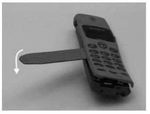
5. Push the hook release jig gently to the lower side, while holding the CMD-C1. In this way the hook release jig is used as a lever. More clamps between upper and lower case will now release and the parts can be taken out.
