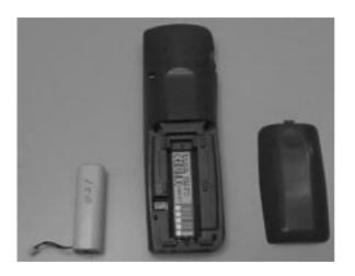
1. Remove the battery cover and the battery. Note that the SIM card is also located in this area.
