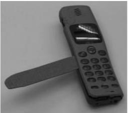
4. Insert the hook release jig (p/n 9-948-370-20) in the gap between upper and lower cosmetic, as indicated in the picture.
